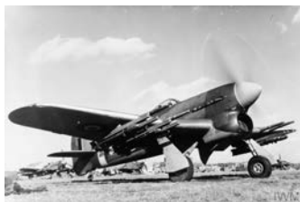
Typhoon Mk 1B SF-T of 137 Squadron with full load of 60 pound rockets on B78 Eindhoven airfield
